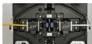
Pigtail to drop cable
